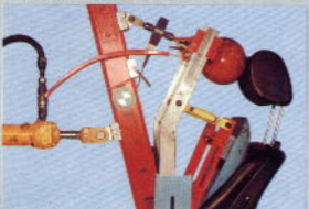
Load-testing the integrated seat belt fixture.
