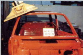
Testing the strength of roof and the over-top - safety structure.
