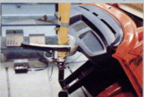
Repeatable impact test on the instrument, energy-absorbing gear, and steering wheel.
