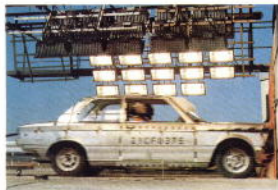
Crash tests to optimize the deformation behavior of the front and rear vehicle ends.
