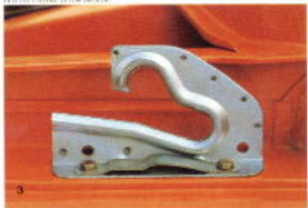
Search for the locking system with safety hooks.
