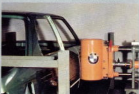
Testing the strength of a side door.
