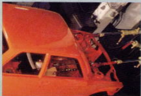
Strength tests on the front panel, the roof, and seat belt anchoring points.
