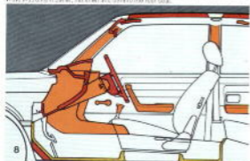
The interior design is based around structural safety features - the instrument panel continue being air-deflectors.
